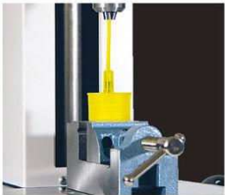
Insert test of plastic pipe
