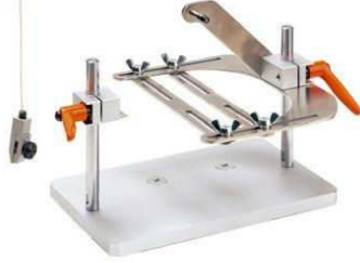
Peeling test of food contain cup
