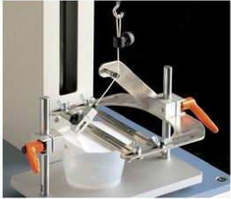
Peeling test of food contain cup
