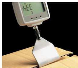
Opening strength of glued corrugated cardboard
