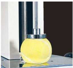
Compression test of tennis ball
