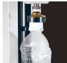
Compression test of plastic bottle
