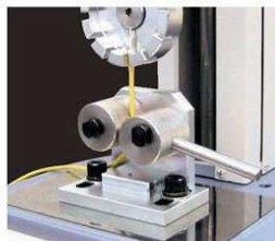
Wire harness strength test
