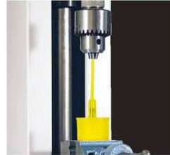
Insert test of plastic pipe
