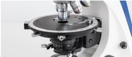
Center-adjustable and turnable polarisation stage
