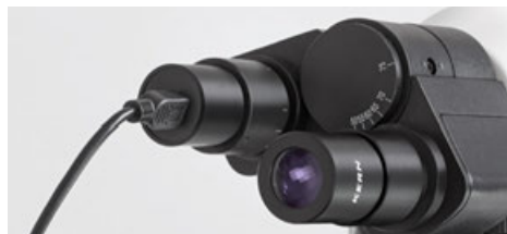
Eyepiece camera fixed into the tube
