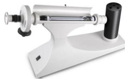
Cuvette in measuring chamber
