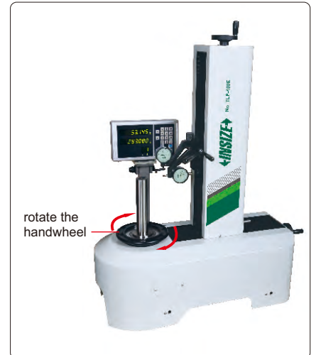
rotate the handwheel to rotate tools
