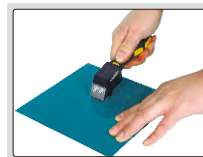
step 1: make grid cutting on surface
